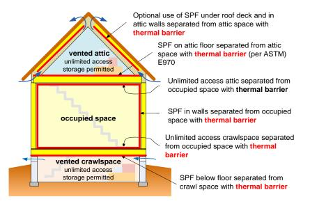
FIGURE C4 – Thermal barrier requirements for vented attics and crawlspaces with unlimited access
