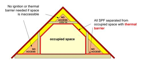
FIGURE C5 – Thermal barrier requirements for areas having no access adjacent to occupied spaces
