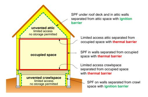
FIGURE C1 – Thermal and ignition barrier requirements for unvented attics and crawlspaces having limited access and no storage
