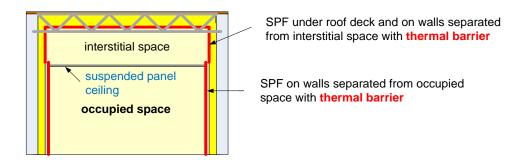
FIGURE C6 – Thermal barrier requirements for interstitial space with suspended panel ceilings which are not thermal barriers
