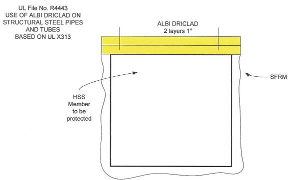
Wall thickness of HSS must be 5/16" minimum
