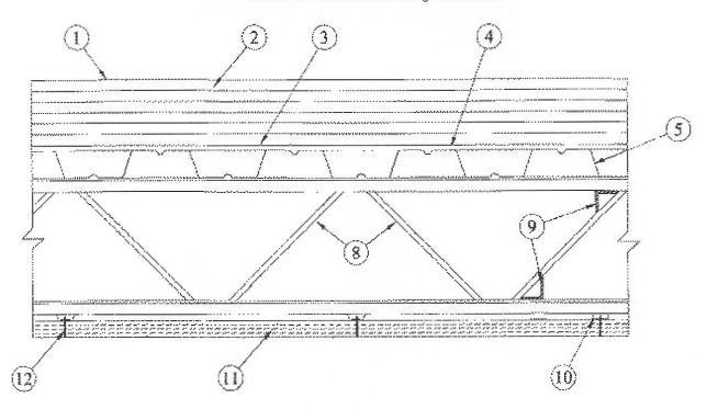
1. **Roof Covering\*** — Consisting of hot mopped or cold application materials compatible with insulation(s) described herein which provide Class A, B or C coverings.
