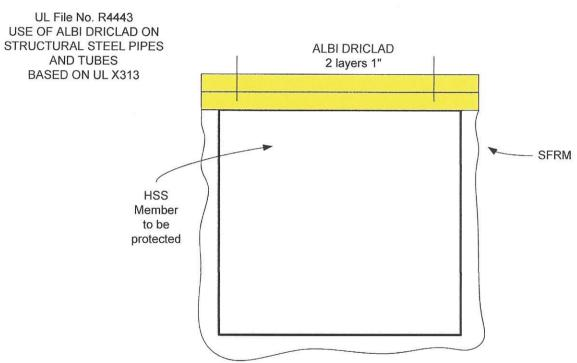
Wall thickness of HSS must be 5/16" minimum
